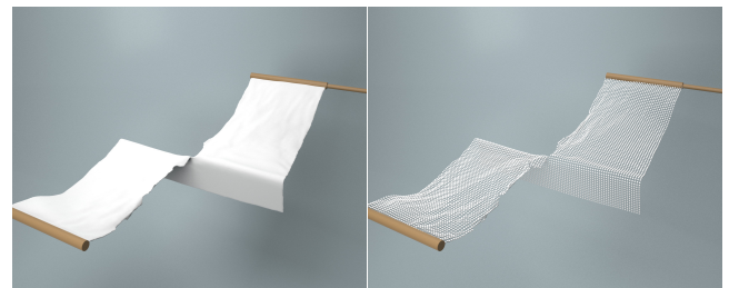
Figure 12: Comparison between particles and mesh. (Left) Surface mesh generated by Houdini [Std20]. (Right) Raw data of particles. Our raw data of particles provides more realistic details of cracks along the tear and the subtle wrinkles on the membrane surface, which the mesh generated by Houdini fails to capture.
