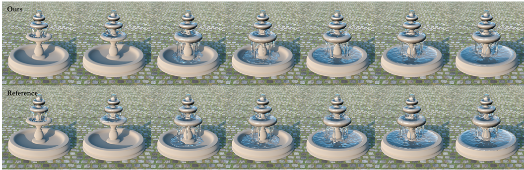
Fig. 2. The characteristic pattern of liquid flowing down a fountain. (Top) Our generalized constitutive model using \kappa > 0, \mu = 0, \eta = 0 and no viscoplasticity or elastoplasticity. (Bottom) Reference results using the equation-of-state fluid model.
