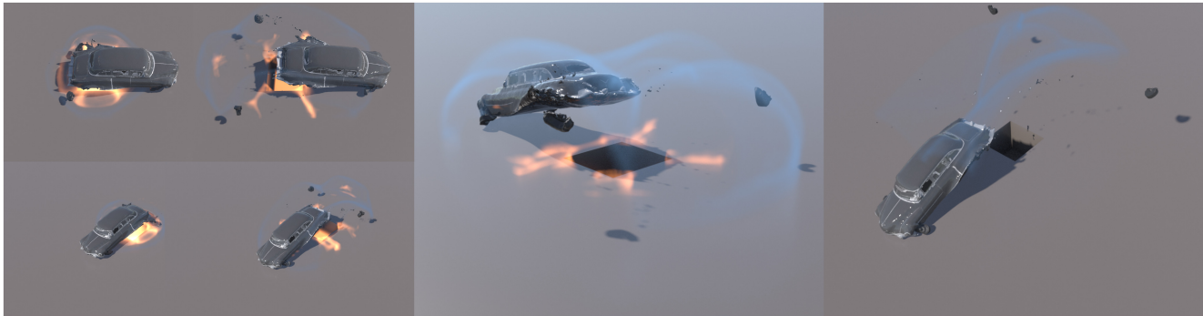
Fig. 1. A car drives through a triggered landmine. The body and the wheels are made of different materials, leading to their distinctive interactions with the blowing exhaust. Our method naturally captures the corresponding effects and solves the solid-gas coupling problem in a monolithic style.
